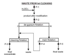
Figure 2. Diagram of enrichment with marked points of sample collection
