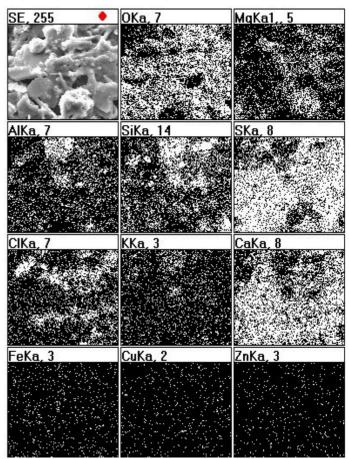
Figure 3. EDS map of particular elements distribution in the selected area of sample P-2
