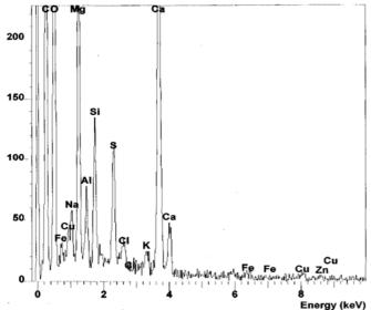
Figure 5. EDS plot showing the presence of particular elements distribution in an analyzed spot of sample P-2
